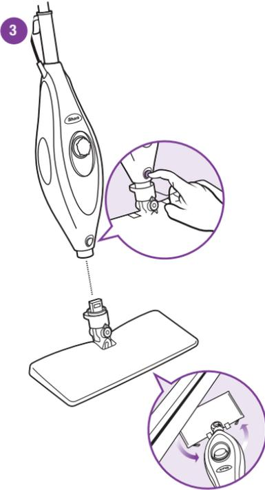
**3** Snap the mop head into the mop body until you hear it latch into place. To release the mop head, press the release button located at the connection of the mop head and the unit.
