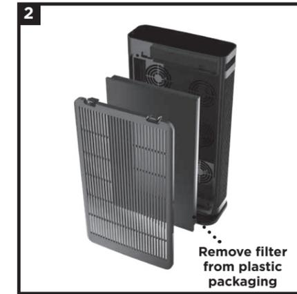
Take the filter out of its packaging, then insert it back into the unit. **DO NOT** run the air purifier unless the filter is removed from its packaging and properly reinstalled.
