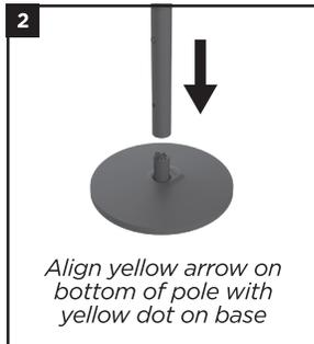
2. Align the yellow dot on the assembled pole with the yellow arrow on the **Base**, then slide the pole down onto the base. Ensure that the pole is fully against the base before proceeding.
