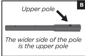
1. Align and insert the **Upper Pole** into the **Lower Pole** until it clicks into place.
