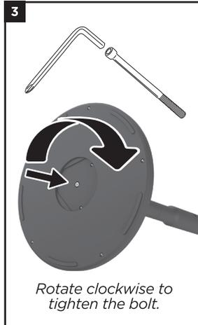
3. Insert the **Bolt** in the bottom of the **Base**. Use the **Allen Wrench** to turn the bolt clockwise to fasten it to the assembled pole.
