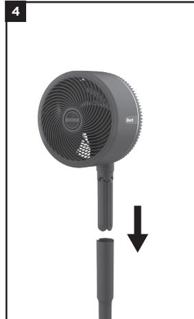
4. **CAUTION:** finger pinch risk. Holding it by the handle, insert the fan head into the top of the assembled pole until it clicks into place.
