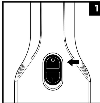
1. Make sure to switch the unit into the "O" position to power off before charging.
