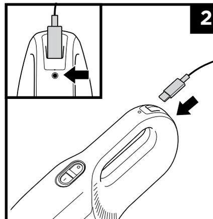
2. Plug the USB-C end of the charging cord into the port on the handle. Plug the USB end of the charging cord into a compatible USB outlet cube or adaptor (not included) and plug into a wall outlet.
