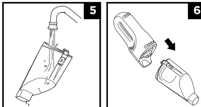
5. To clean the interior of the dust cup, rinse it with water. Place it on its side with the lid open to air-dry for at least 24-48 hours before reinstalling.
