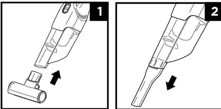
1. To install an accessory, align it with the nozzle, then slide it on.
