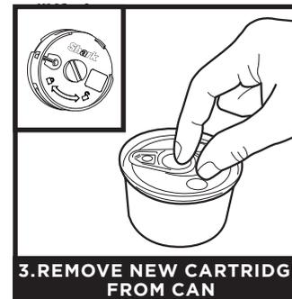
Remove the new cartridge from the can. To maintain the life of the cartridge, keep it in the can until you are ready to install it.
