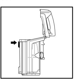
To remove collected debris from **Lint Screen**, press top release button and lift handle to access screen. Gently brush lint screen to clean.
