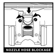
To access the nozzle hose, open the locks on the bottom of the nozzle. With a coin, turn the locks counterclockwise, then lift the cover and clear any blockages.
