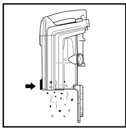
To empty debris into trash, press lower release button and bottom of dust cup will drop open.
