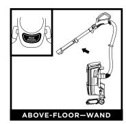
Press the **Wand Release** button to detach the wand from the pod.
