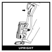
To engage brushrolls, turn on power, then step on floor nozzle and tilt handle back.
