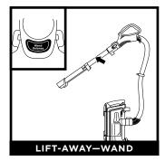
With pod removed, press the Wand Release button to detach the wand from the floor nozzle.
