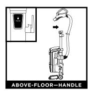
Press the **Handle** button to detach the handle from the wand.
