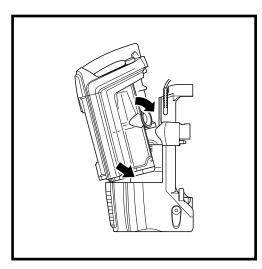
To reinstall, place bottom of dust cup into pod and then tilt the dust cup until it clicks into place.
