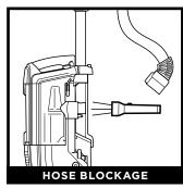
Detach hose from vacuum pod, and check hose and opening on back of pod for blockages.
