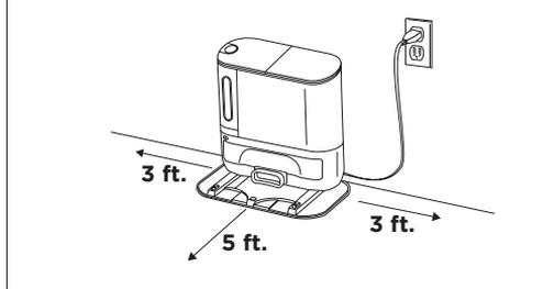
Find a **permanent** location for the base. Place it with its back against a wall, in an area with a strong Wi-Fi signal. **Remove any objects** that are closer than 3 ft. from either side of the base, or closer than 5 ft. from the front. For best results, set up base on **bare floor**.
