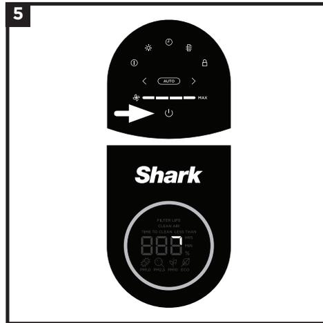
5. Plug the unit into an electrical outlet and press the power button on the top control panel. When the unit is powered on, it will begin to analyze the air quality indicated by the rotating lights. After a few seconds, the unit will display the current air quality
