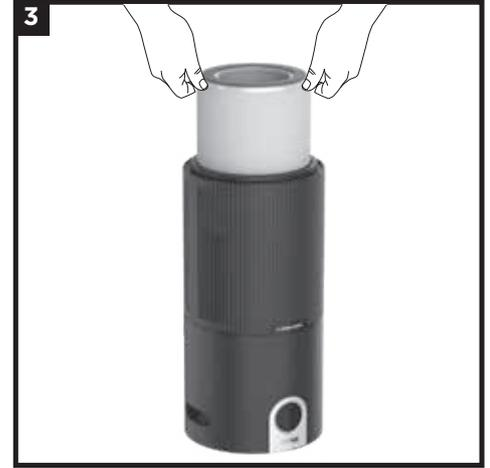
2. With the filter reinstalled, twist the filter door until it clicks into place.
