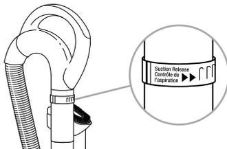
This vacuum has huge suction power. The suction can be adjusted to make the vacuum easier to push and pull on certain types of carpets as needed.
