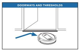
Your robot can easily climb over most thresholds, but if one is higher than an inch, block it off with a BotBoundary<sup>®</sup> strip.
