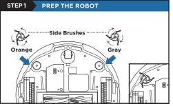
Snap the 2 side brushes onto the pegs on the bottom of the robot. When installed correctly, the orange brush will spin counterclockwise and the gray brush will spin clockwise. The side brushes are located in the red packaging.
