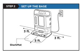
Find a permanent location for the base. Place it with its back against a wall, in an area with a good Wi-Fi signal. Remove any objects that are closer than 3 ft. from either side or closer than 5 ft. from the front.
