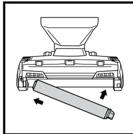
To remove the **Soft Roller** from the nozzle, lift it out by the pull tab. Tap loose debris off the Soft Roller. Use a dry towel to wipe the Soft Roller clean, or to remove any debris caught in the teeth behind the Soft Roller.
