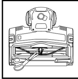
To open the brushroll garage, slide both release buttons on the floor nozzle away from you, towards the back of the nozzle, then lift off the lid. Clear away any objects or debris.
