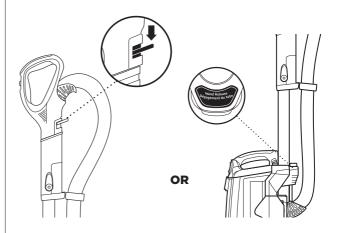
1 Press the Handle Release OR Press the Wand Release button when you need to clean within short reach.
