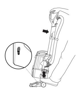
Plug power cord into outlet. Place foot on floor nozzle and tilt handle back.
