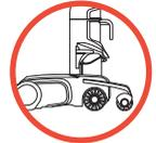
When the vacuum is placed in the upright position, the retractable wheels will extend so the vacuum can stand up on its own.
