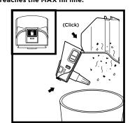
Hold the dust cup over the trash. Press the **Empty** button and pull open the dust cup lid until it clicks and locks in the open position. Gently tap the cone-shaped screen inside the dust cup to knock dust and debris into the trash.
