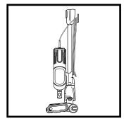
Wrap the cord around the two cord hooks. Start with the top hook, and leave a little slack in the cord.
