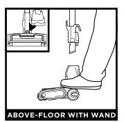
For more reach, detach the wand. Stand the vacuum upright, step on the **Foot Pedal** on the side of the nozzle, and pull up the wand to detach.
