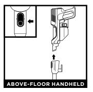
To detach the handheld vacuum, press the **Wand Release** button and lift the handheld vacuum off the wand. Great for cleaning stairs, furniture, and countertops.
