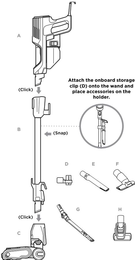
**NOTE: For proper operation, ensure all parts are firmly CLICKED into place.**
