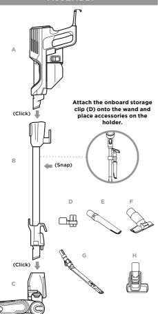
NOTE: For proper operation, ensure all parts are firmly CLICKED into place.
