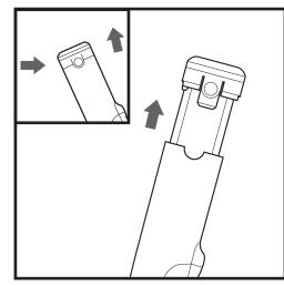
To remove the battery from the hand vacuum, press the release tabs on the battery cap and slide the battery out.
