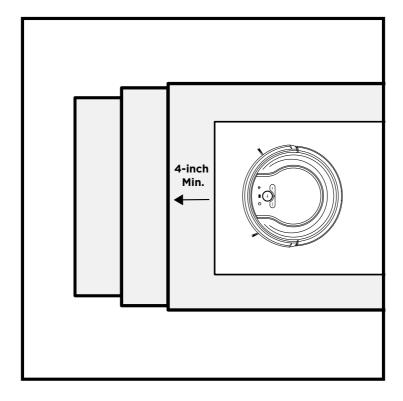
For your robot's cliff sensors to work properly, all runners, rugs, or carpets must be at least 4 inches from the top of any stairs (or extend over the edge of the stairs.)
