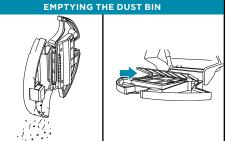
During the first few weeks of use, the dust bin will need to be emptied more frequently, as your robot will now be removing dust and debris from areas that were previously hard to reach. Empty debris and dust into trash.
