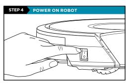
To charge, the **Power** button on the side of the robot must be in the ON position (I).
