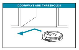
Your robot can easily climb over most thresholds, but if one is too high, set up a no-go zone in the app to block it off.
