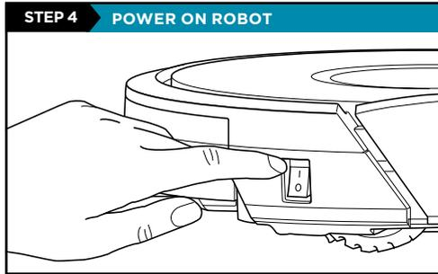
To charge, the **Power** button on the side of the robot must be in the ON position (I).
