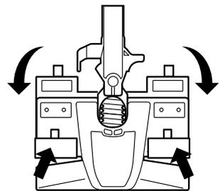
**2** Pull the other two tabs tightly around to the back fasteners. Ensure the pad is flat against the bottom surface and tightly secured.
