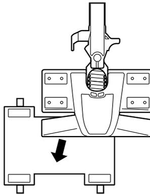
**1** Slip two tabs between the nozzle and the cluster base and attach them to the front fasteners.
