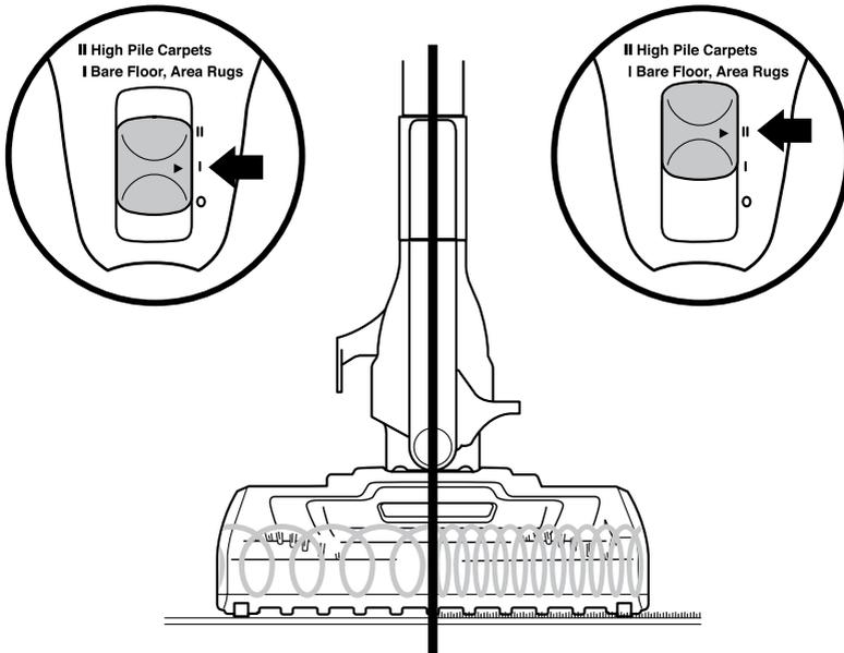
The Rocket® Deluxe Pro Ultra-Light has a 2-speed power slider switch on the handle. Slide the power switch to appropriate speed setting (I or II) and start cleaning.
