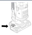
The motorized brush indicator light will illuminate Green when motorized floor brush is on. If there is a blockage or jam, the light will turn Red.
