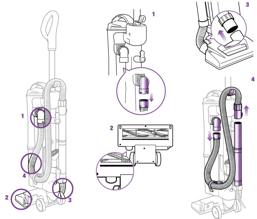
Blockages may cause your vacuum to overheat and shut down. If so, clear the blockages, then follow the instructions for Resetting the Motor Thermostat on page 13.
