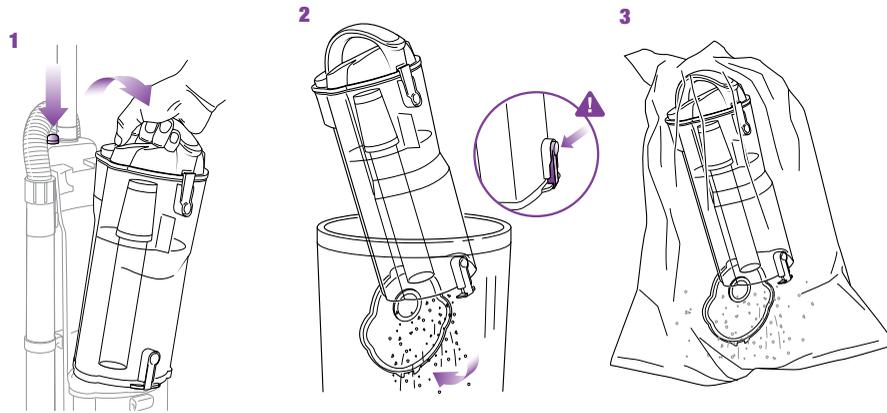
For best results empty the Dust Cup after each use; empty several times during prolonged usage, or when it reaches the **MAX** fill line. **NEVER OVER-FILL THE DUST CUP.** Stand vacuum into upright position. Turn vacuum off.
