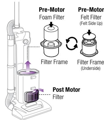
**⚠ IMPORTANT:** Loss of Suction may occur if filters are not cleaned every 3 months. Rinse and allow to air dry completely. Tap loose dirt from foam filter as needed in between washing. Filters may appear dirty after use - this is normal.
