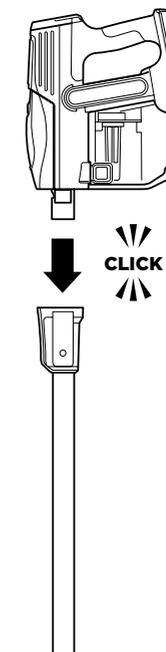
**1** Insert the wand into the floor nozzle, pressing it in until it clicks securely into place.
