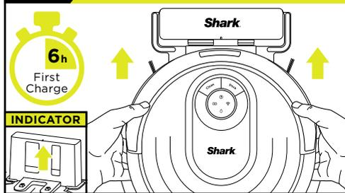
Place robot on dock to charge. The dock indicator light will turn **blue** and the robot will beep when charging begins.
