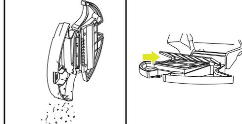
During the first few weeks of use, the dust bin will need to be emptied more frequently, as the robot cleans areas that were previously hard to reach. Empty debris and dust into trash. Remove any debris between the filter and the plastic shield.
