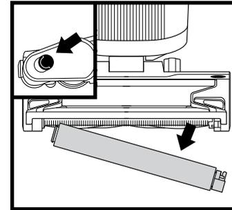
Slide the Soft Roller access button forward to release the Soft Roller.
