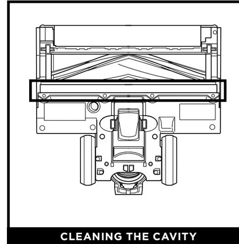
1. With the strip removed, clean the squeegee cavity and bristle strip. Use a paper towel to wipe off any debris or dust in the cavity and on the bristle strip.
