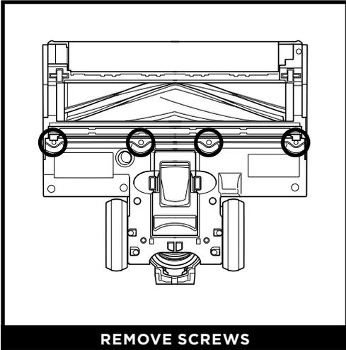
1. Turn the nozzle over and locate the squeegee bristle strip between the brushroll and the rear wheels. Use a Phillips-head screwdriver to remove the 4 screws.
