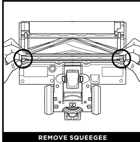
2. Remove the squeegee strip by pulling up on the fabric flaps on both ends of the strip.
