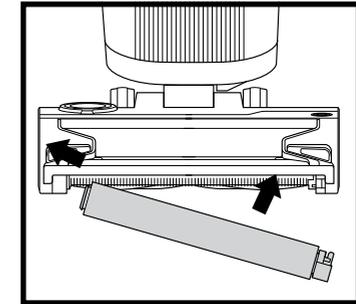
Hand wash the Soft Roller as needed. Use only water, and allow it to air-dry completely for at least 24 hours. Reinsert the Soft Roller in the front of the nozzle until it clicks into place.
