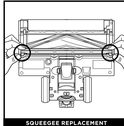
1. Hold the squeegee strip by the fabric flaps on the ends, with the bristle side facing up. Insert the plastic piece into the cavity first, while tilting the strip forward, toward the brushroll.
