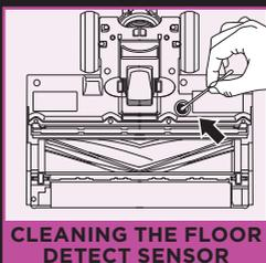
CLEANING THE FLOOR DETECT SENSOR
