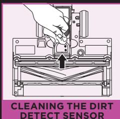
CLEANING THE DIRT DETECT SENSOR
