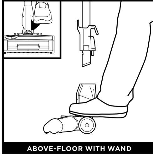
For more reach, detach the wand. Stand the vacuum upright, step on the **Foot Pedal** on the side of the nozzle, and pull up the wand to detach.
