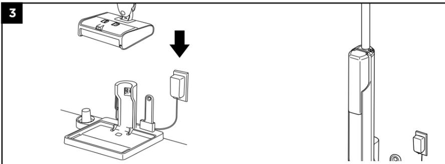
3. Charge the unit by placing it on the **Charging Dock**. Make sure the contacts on the body are aligned with the contacts on the charging dock. The LEDs on the main body will illuminate when charging begins.
