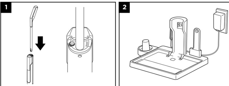
1. Align the **Pole** with the opening in the Main Body and insert firmly until it clicks into place.
