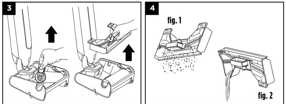
3. Grip the side tab and lift out the **Brushroll**, then remove the **Debris Holder** by pulling up on the handle. 4. First, dump out solid waste (**fig. 1**) then open the pull tab and pour out liquid waste (**fig. 2**).
