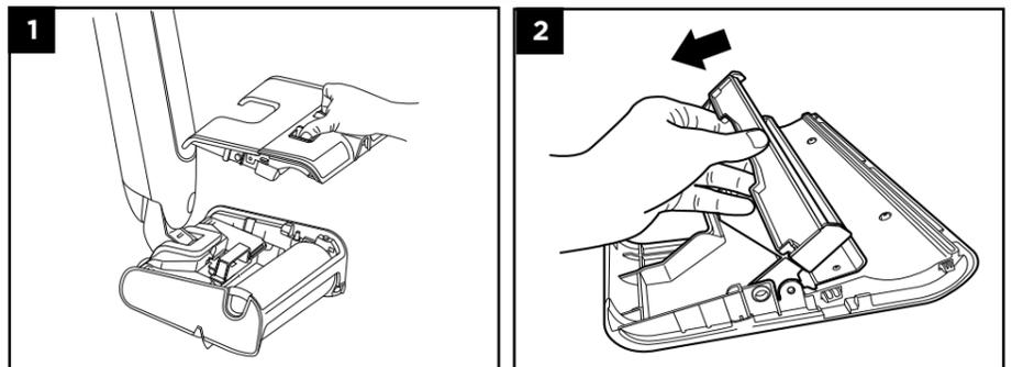
1. Remove the **Nozzle Cover**: Press both tabs and lift off the cover. 2. Hold the cover over a sink or trash bin, then carefully turn it over to dump out waste. Pull back the **Debris Plate** to clean off any remaining liquid and debris.
