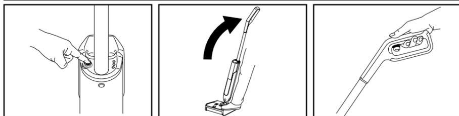
1. Press the Power button. 2. Lower the handle to activate the brushroll and debris illumination light. 3. Press the trigger to spray.
