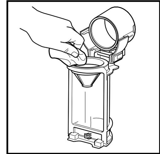
To deep-clean the dust cup, slide the release button until the lid opens completely. Wipe away any dust and debris with a dry cloth, then rinse it out with water. Use a damp cloth to remove any remaining debris. Allow the dust cup to air-dry completely for at least 24 hours before reinstalling it.
