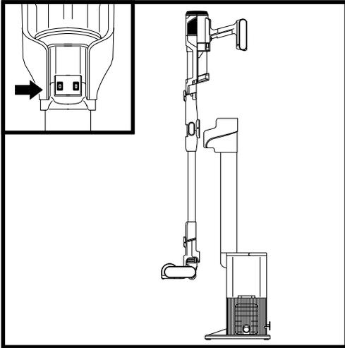
Place the vacuum on the dock in a downward motion. Once properly attached, the auto evacuation process will begin. The evacuation cycle will last for 10 seconds.
