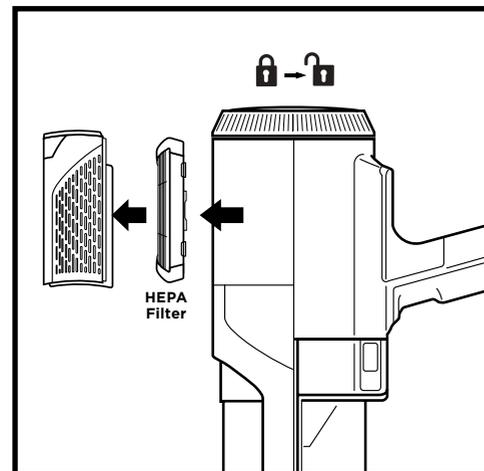
1. To access the HEPA filter, rotate the filter cover on the handheld vacuum to the unlocked position.
