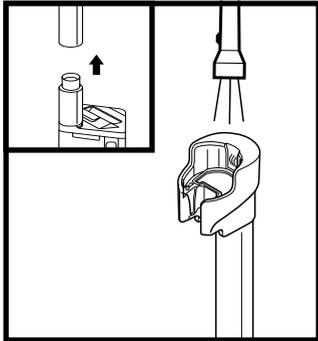
Checking for Blockages in the Charging Post:
