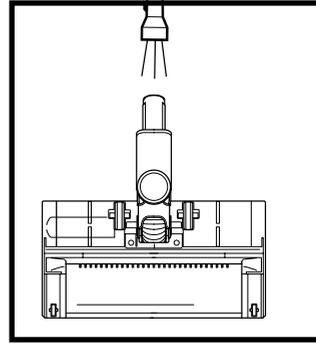
Checking for Blockages in the Floor Nozzle:
