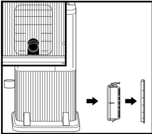
To access the dock filter, remove the filter door. Press the button at the bottom of the door, tilt the door and lift it off, then remove the filter. Rinse the filter with cold water **ONLY**. Do not use soap. Allow the filter to air-dry completely, then reinstall it by reinserting it into the dock and replacing the filter door.
