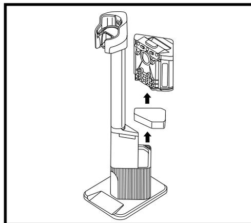
To access the foam exhaust filter in the dock, first remove the dust bin, then vacuum off any fine dust or debris from the filter. Lift the foam filter out of the dock, then rinse it with water only-- do not use soap. Allow the foam filter to air-dry completely before reinstalling it.
