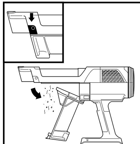
To empty the handheld vacuum (IW4615 Series) dust cup, turn off the power and hold the hand vac over the trash. Press the release button and the dust cup lid will drop open, releasing debris.
