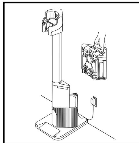
The dock dust bin holds up to 30 days' worth of dust and debris. To remove the bin, lift it out by the handle.
