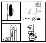
To put the vacuum in storage mode, press the unlock latch while folding the handheld vacuum forward until the wand clicks and locks.
