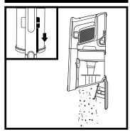
To empty the **Dust Cup** while it is attached to the handheld vacuum, position the dust cup over a trash receptacle and slide the **CleanTouch\* Lid Release** slider forward.
