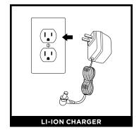
Plug the **Li-Ion Charger** into a wall outlet.
