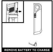
Press and hold the **Battery Release Button**, then slide out the battery. Plug the charger into the charging port on the battery. To reinstall the battery, slide it into the slot in the back of the handheld vacuum.
