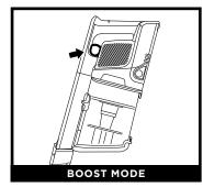
For an added boost in power, pull the **Trigger** on the handheld vacuum. Release it to return to standard power.
