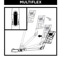
Press the **MulitFLEX Wand Unlock Latch** on the back of the wand, then adjust the angle for cleaning under furniture.
