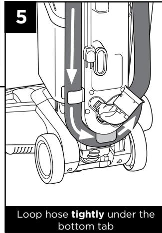
Loop hose **tightly** under the bottom tab
