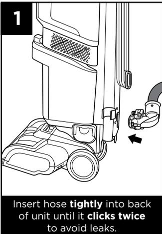
Insert hose **tightly** into back of unit until it **clicks twice** to avoid leaks.
