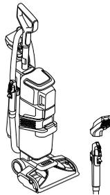
**Tip:** For improved suction, tilt the angle of the tool forward (**fig. 9**). More extracted liquid will appear in the window on the tool as suction increases.
