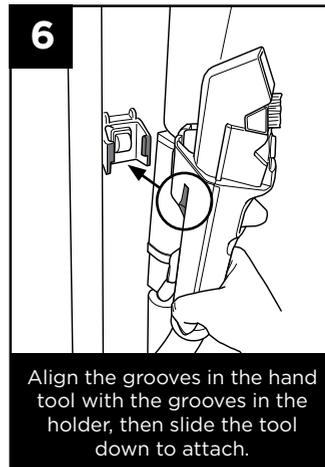
Align the grooves in the hand tool with the grooves in the holder, then slide the tool down to attach.
